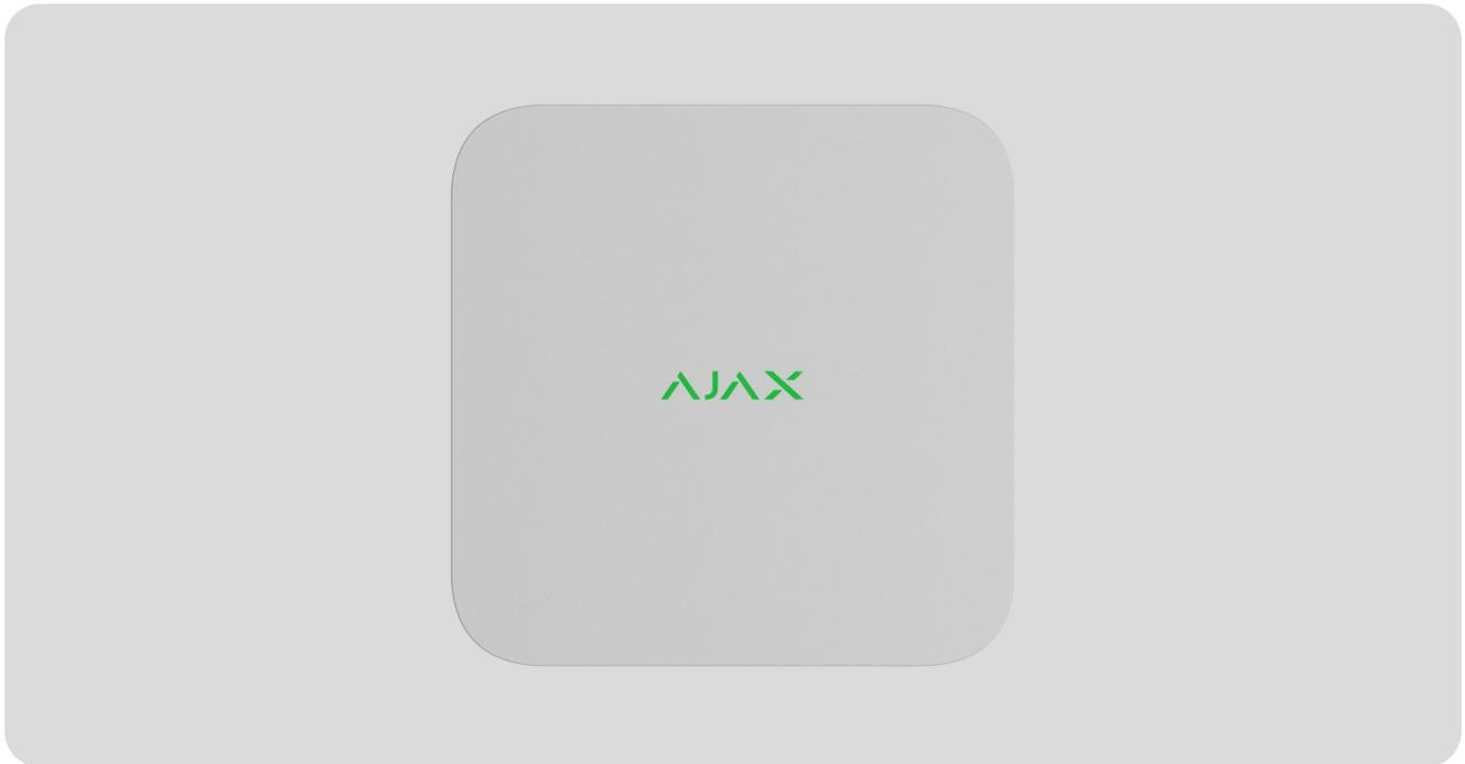
**NVR** is a network video recorder for home and office video surveillance. You can connect third-party IP cameras to the device.
